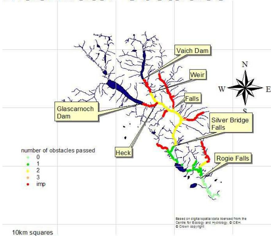
The fish ladder at Rogie is well designed and allows fish to ascend at a wide range of flows. However in very low flows Rogie Falls can delay migrating salmon and the pools downstream are especially vulnerable to poaching. Glascarnoch and Vaich Dams have no provision for fish passage and cut off the headwaters of the system. A weir constructed in Strath Vaich restricts trout movement but also modifies habitats upstream and could be removed as it no longer fulfils a function.
