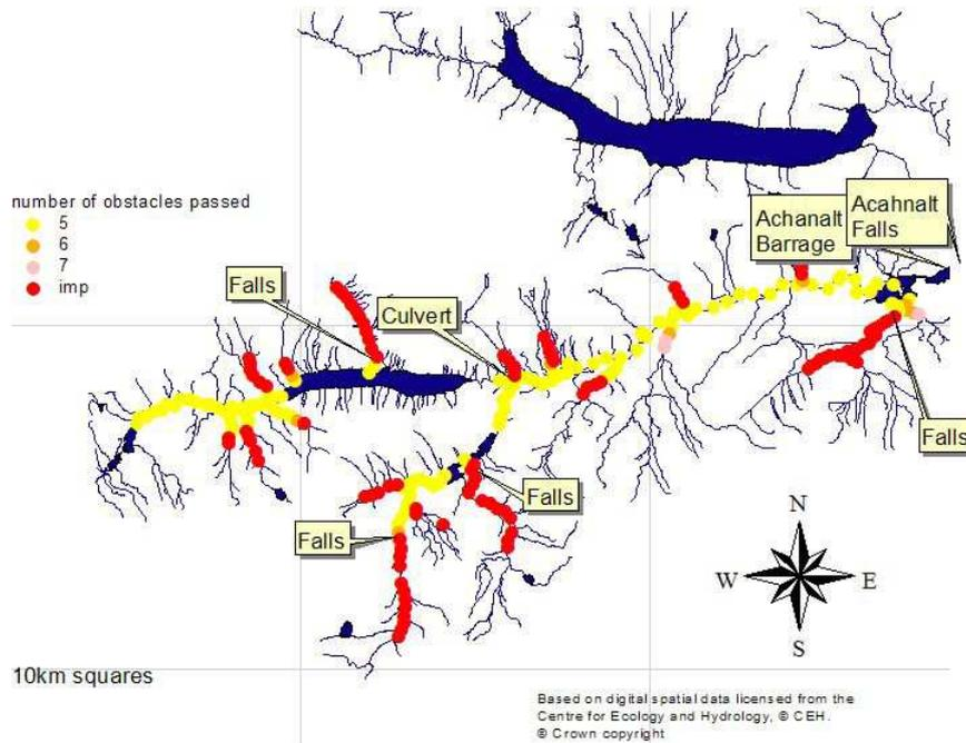
The fish ladder at Achanalt was modified as a result of radio-tracking work to improve its performance. There is still an increased risk of predation by otters and of poaching below the ladder. The small Borland Lift in the centre of Achanalt Barrage may allow some fish to pass upstream but it is equally likely that fish will pass under the Barrage gates which are opened even after moderate rainfall.
