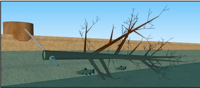
Picture 3. Two Diagrams illustrating how the sycamore were felled in situ before being wired to their stumps. Diagram courtesy of WTT.
