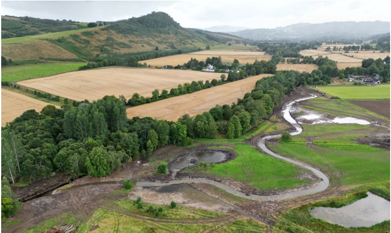
Figure 4: Re-meandering of the River Peffery at Fodderty. You can see the channelised burn as it enters the trees (far left). Photo courtesy of Lockett Agrienvironment (2022).
